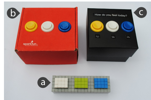
Figure 2. Voting devices: a) lo-fi Lego prototype, b) hi-fi prototype, c) final version.
